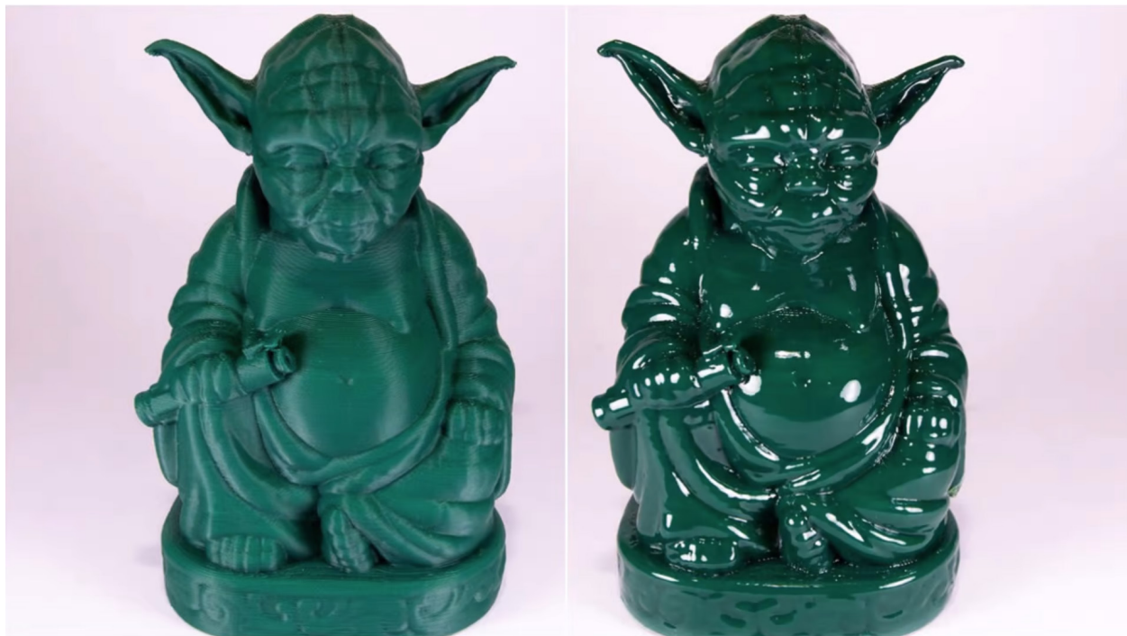
Effects of vapor smoothing of ABS
