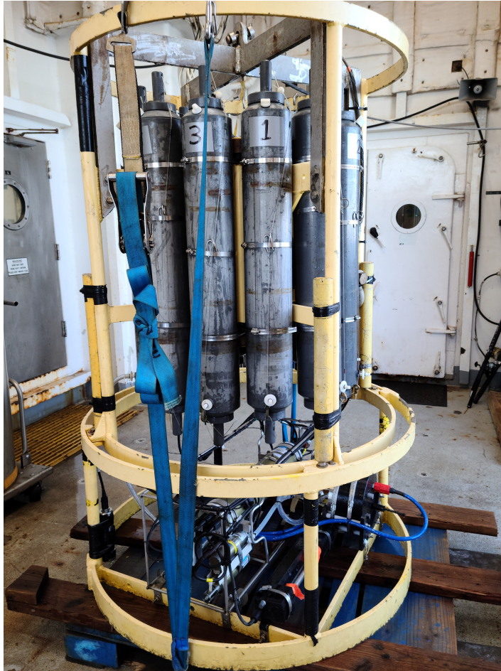
Figure 2.5: CTD Rosette . A picture of the rosette on R/V Revelle during RR2107 activities.
