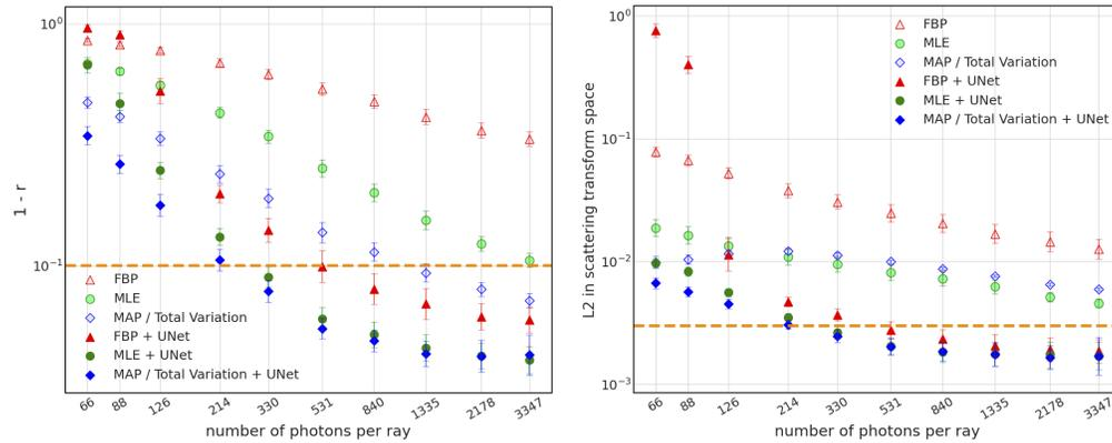
**Fig. 7.** Quantitative comparison between different reconstruction algorithms for experimental data of 40 instances under different photon counts per ray. Symbols and error bars as in Fig. 5. The dotted orange lines show the thresholds of acceptable performance.
