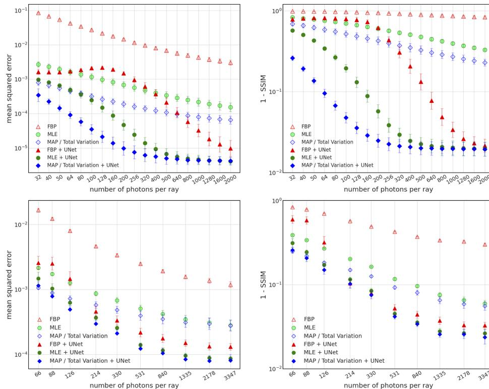
**Fig. 8.** Quantitative comparison between different reconstruction algorithms with mean squared error (MSE) and structural similarity index measure (SSIM) metrics. The top two figures are for simulated data, and the bottom two are for experimental results.
