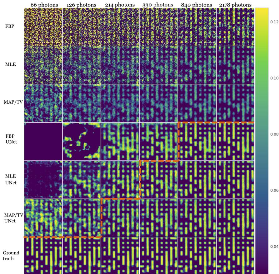
**Fig. 6.** Selected 2D reconstructions (in  $128 \times 128$ ) for different algorithms using experimental data. Each row represents a reconstruction algorithm. Each column represents an intensity of the photon rays. The dotted orange line is the boundary between acceptable and unacceptable performance as determined by the MST metric.
