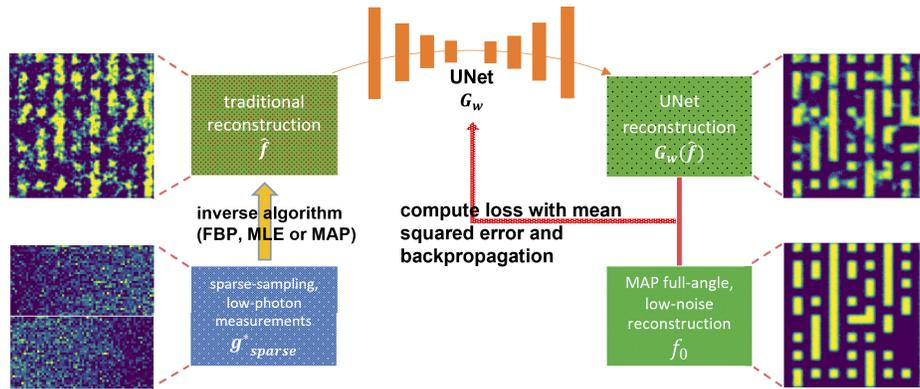
**Fig. 2.** A conceptual diagram for the learning-based algorithms. An inverse algorithm first produces the traditional reconstruction  $\hat{f}$  from the sparsely-sampled and low photon measurements. Then the UNet takes  $\hat{f}$  and outputs reconstruction  $G_w(\hat{f})$ . The differences between  $G_w(\hat{f})$  and  $f_0$  are backpropagated to find the optimal UNet parameters based on Eq. (7).
