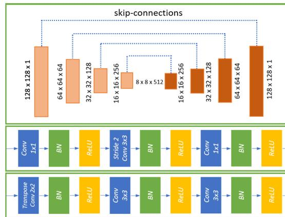
**Fig. 3.** UNet architecture for the learning-based algorithms. The top box shows the overall design of the network, where the light orange modules are downsampling blocks and the dark orange modules are up-sampling blocks. Blue dotted lines represent the skip connections. The middle box shows the design of the downsampling blocks. The bottom box shows the design of up-sampling blocks. BN is batch normalization.
