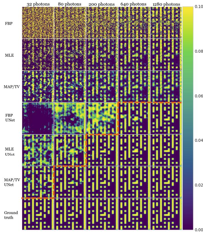
**Fig. 4.** Selected 2D reconstructions (in  $128 \times 128$ ) for different algorithms using simulated data. Each row represents a reconstruction algorithm, and each column represents an intensity of the photon rays. The ground truth is repeated in the last row. The dotted orange line is the boundary between acceptable and unacceptable performance as determined by the MST metric.
