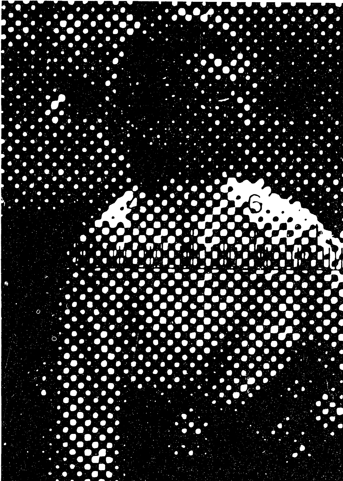
Figure 5.1: Microphotographs of printed classical halftones (continued). (b) Detail from a book published in 1916 [50]. (Reticule is ruled in millimeters.)
