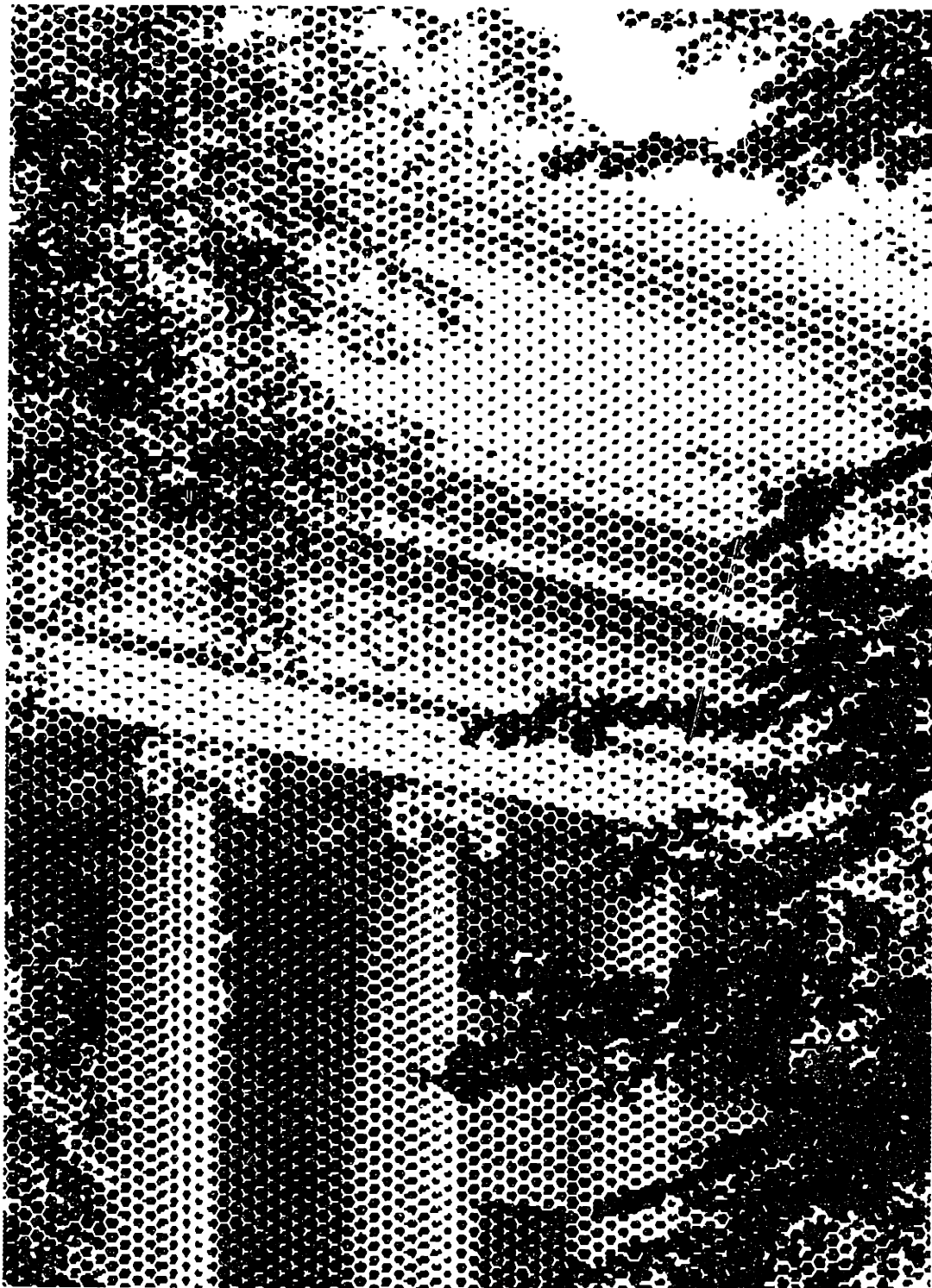
Figure 5.33: Hexagonal Spiral Screen on a Scanned Picture. (28 levels of gray.)
