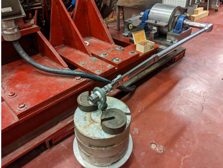
Fig. 15 Heat exchanger loaded to maximum of 857 Nm (112% design torque value of 765 Nm)
