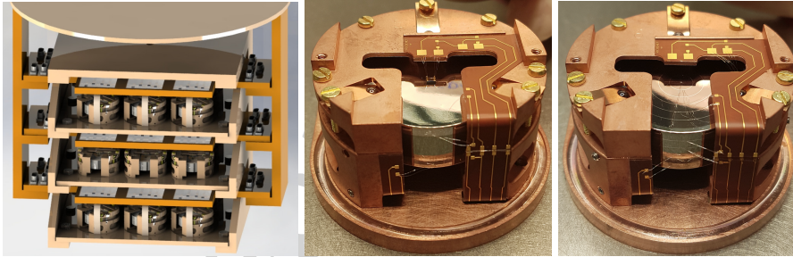
Fig. 4 Left: Draft model of the CryoCube design. All the parts in dark orange correspond to 1 K stage holding the HEMT-based electronics. The light part supports the 27 Ge detectors regulated at about 20 mK. Pictures of a planar (middle) and an FID (right) detector prototype.
