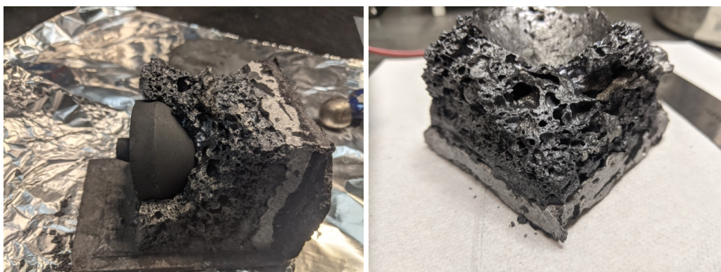
Figure 5 Images of the electrolysis cell following the iron extraction experiment.
