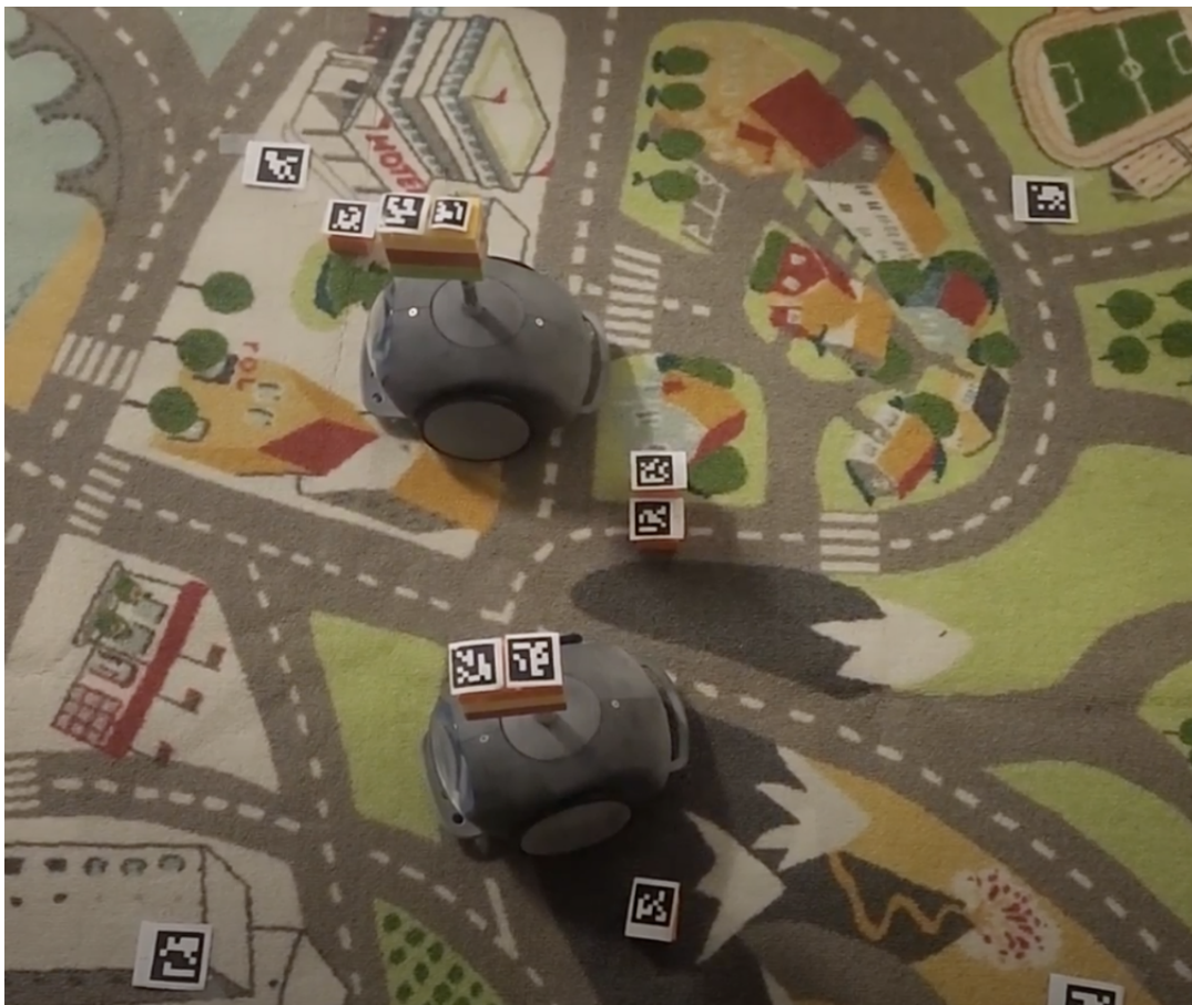
Figure 3-10: View of the playground. Each object is uniquely assigned an Aruco code , which is placed on the top of its body (for the robots) and on one of the Lego pieces' squares (for the rest).
