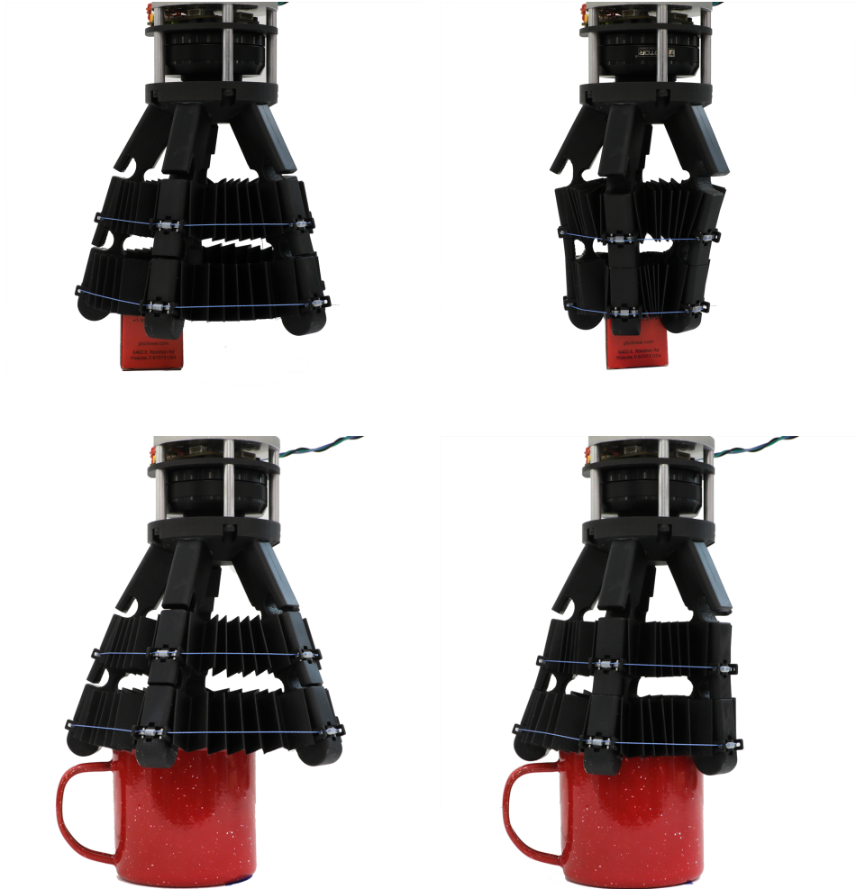
Figure 4-9: Depending on the resistive forces on the grasped object (e.g. friction), FROG’s underactuated structure either cages and centers the object (top) or conforms to the object without object movement (bottom), demonstrating the grippers ability to deal with pose uncertainty.
