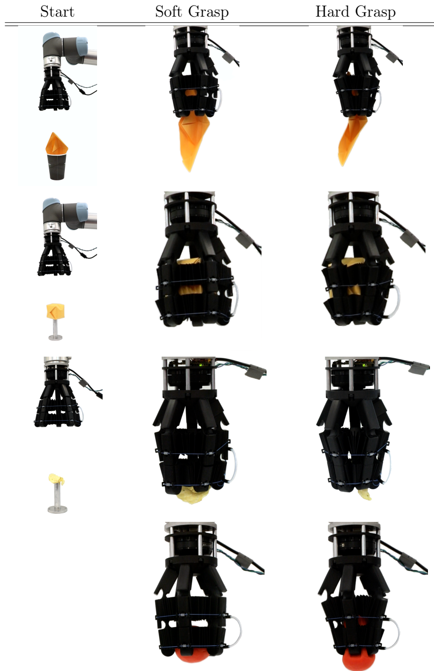
Figure 4-10: FROG’s structure and actuator allow it to easily grasp fragile objects. Columns show start (left), result after a soft grasp (middle), and result after a hard grasp (right). Rows show grasping a paper boat (top), paper ball (top middle), potato chip (bottom middle), and ball of Play-Doh (bottom).
