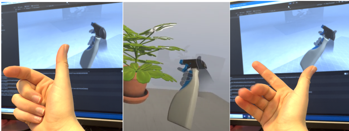
Figure 6-2: Difference between real and virtual hand position when grabbing a virtual object
