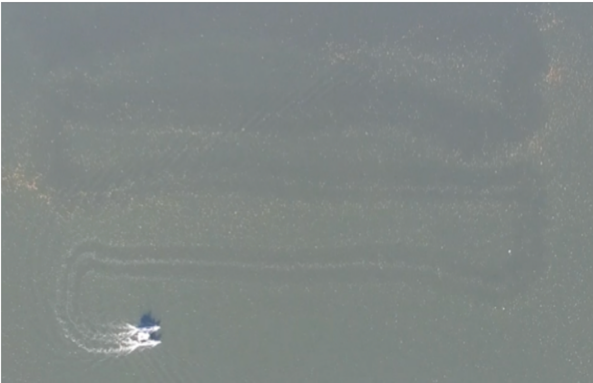
Figure 2-2: Drone photo showing the WAM-V USV operating at the MIT Sailing Pavilion [Bena]. The vehicle uses MOOS-IvP's survey generation capability to patrol an area of the Charles River for demonstration.
