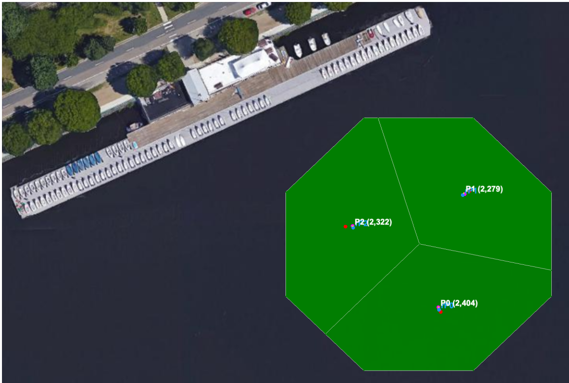
Figure 2-1: An operating area partitioned by the Voronoi algorithm. In this case, every point lying in P1's polygon is closer to P1 than P2 or P3.
