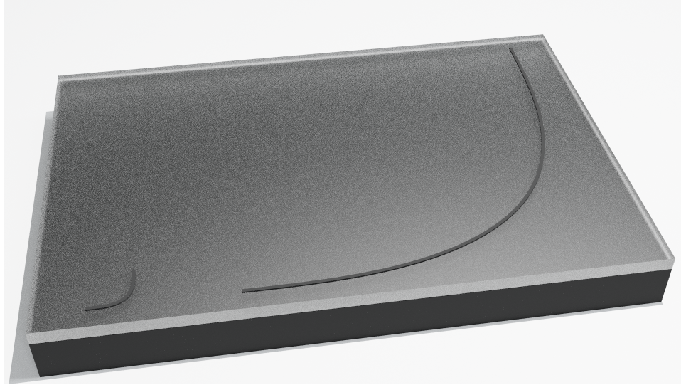
Figure 2-2: Footprint comparison between a 5\ \mu\text{m} radius bend (left), common for dense routing in silicon photonics, vs. a 50\ \mu\text{m} radius bend (right) required for routing on lower index platforms such as lithium niobate and silicon nitride.
