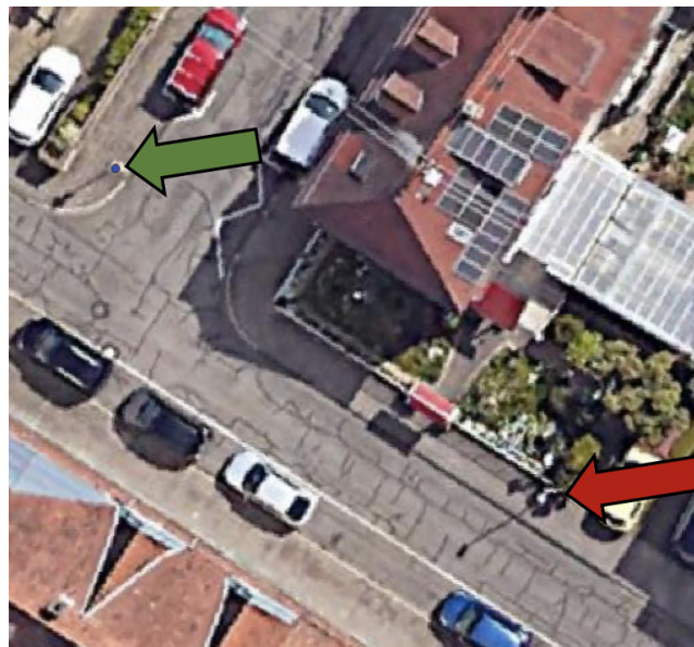
Figure 3-9. Shadows can be used to identify traffic signs in the Google Satellite images. This, however, is unreliable due to lighting and occlusion (see Figure 3-8). Additionally, the difference between traffic signs and street lights is subtle. The traffic sign candidate pointed out by the green arrow is a traffic sign, whereas the candidate identified by the red arrow is not.
