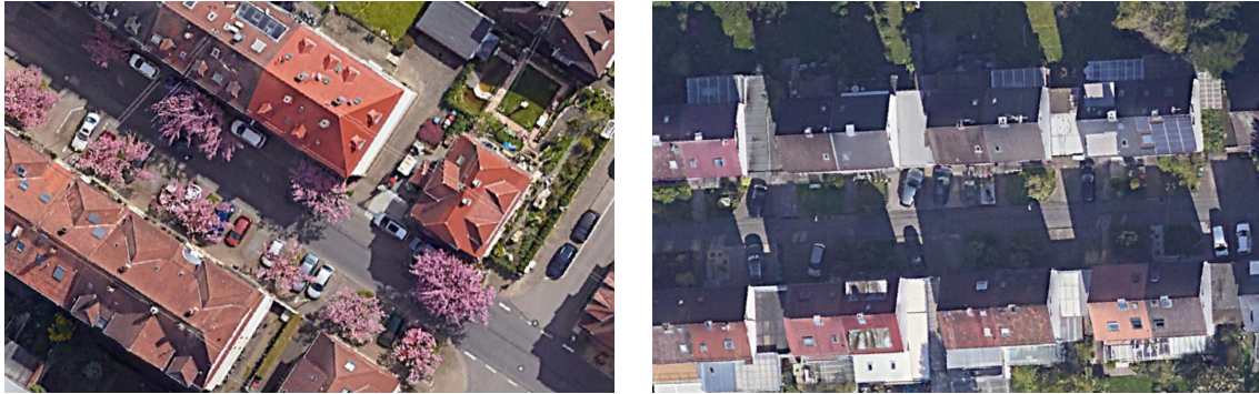
Figure 3-8. Occlusion (left) and lighting (right) in Google Satellite images make identifying cars and traffic signs difficult.
