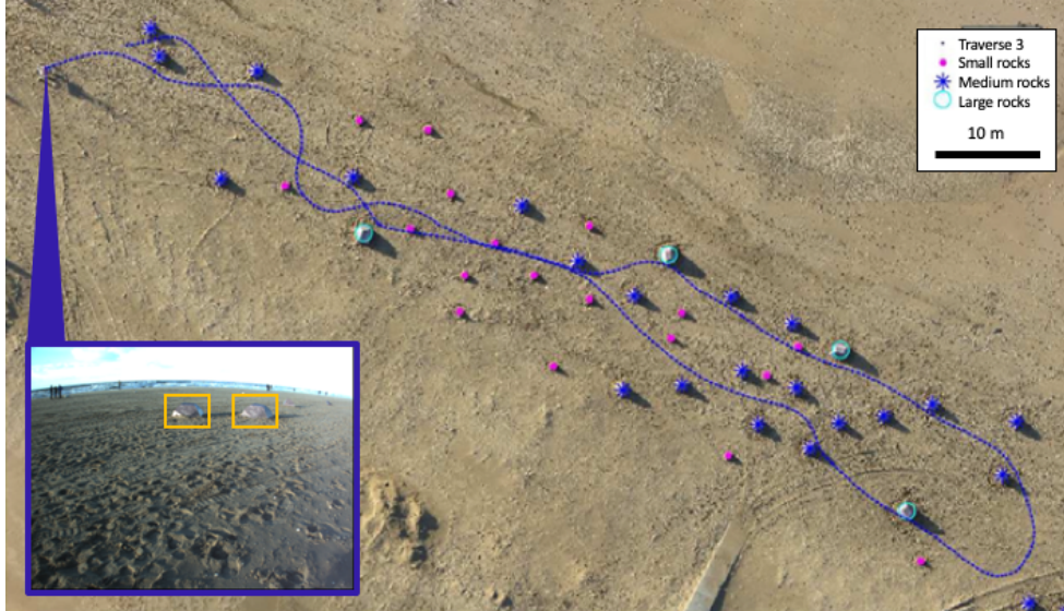
Figure 1-1. The pipeline can localize the ground rover of the Katwijk dataset [17] in an unstructured environment with a ground truth reference map of small, medium, and large rocks. This is accomplished by creating a vehicle object map of the rocks observed while driving (identified by the yellow bounding boxes in image) and registering them with the rocks in the reference map. With a reference map spanning roughly 1 km, 0.68 m accuracy has been achieved on the Katwijk dataset.
