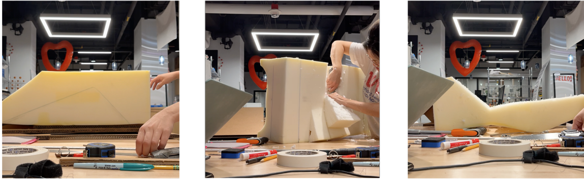
Figure 2-17 - Process of Fabricating Comfort Elevation V0 A) Trace cardboard outline onto foam B) Manually cut out cavity C) Smooth out face
