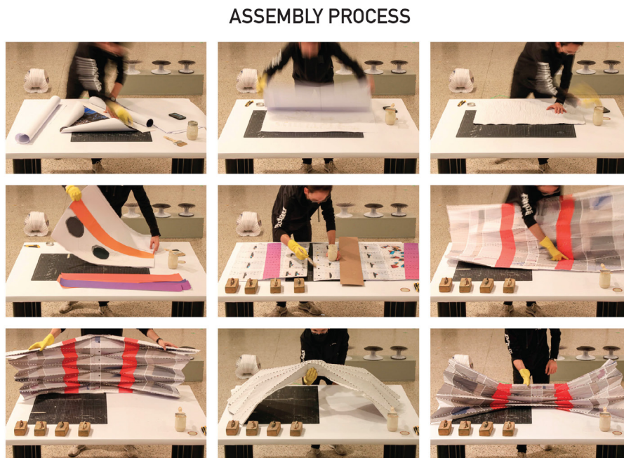
Figure 114 Module fabrication and assembly. Olivier Fabber, 2021. Source: Olivier Fabber, Used with permission of the student
