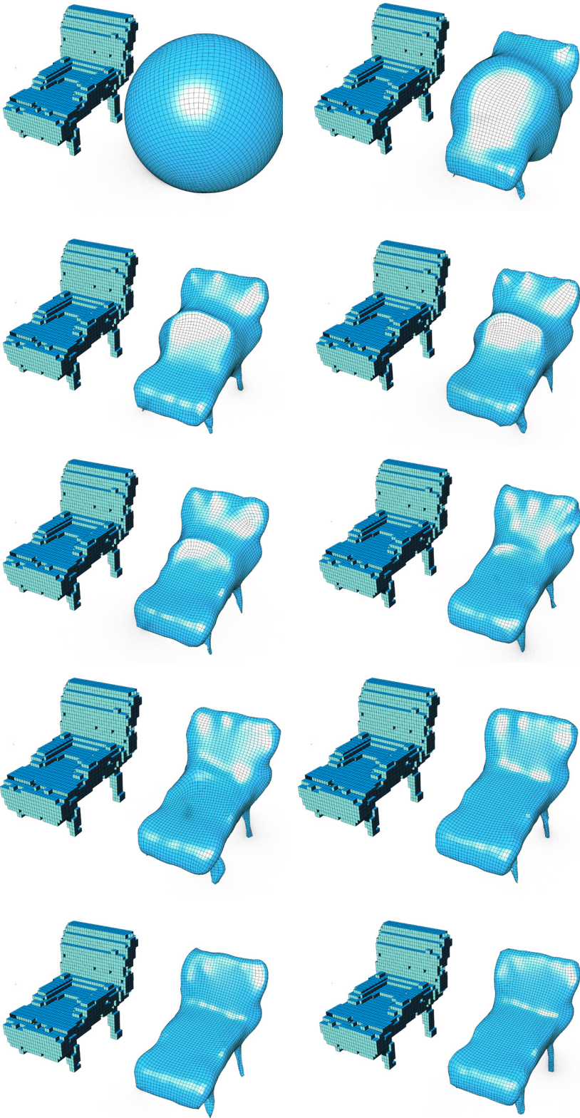
Figure 46 Mesh optimization process using Differential Rendering Source: author
