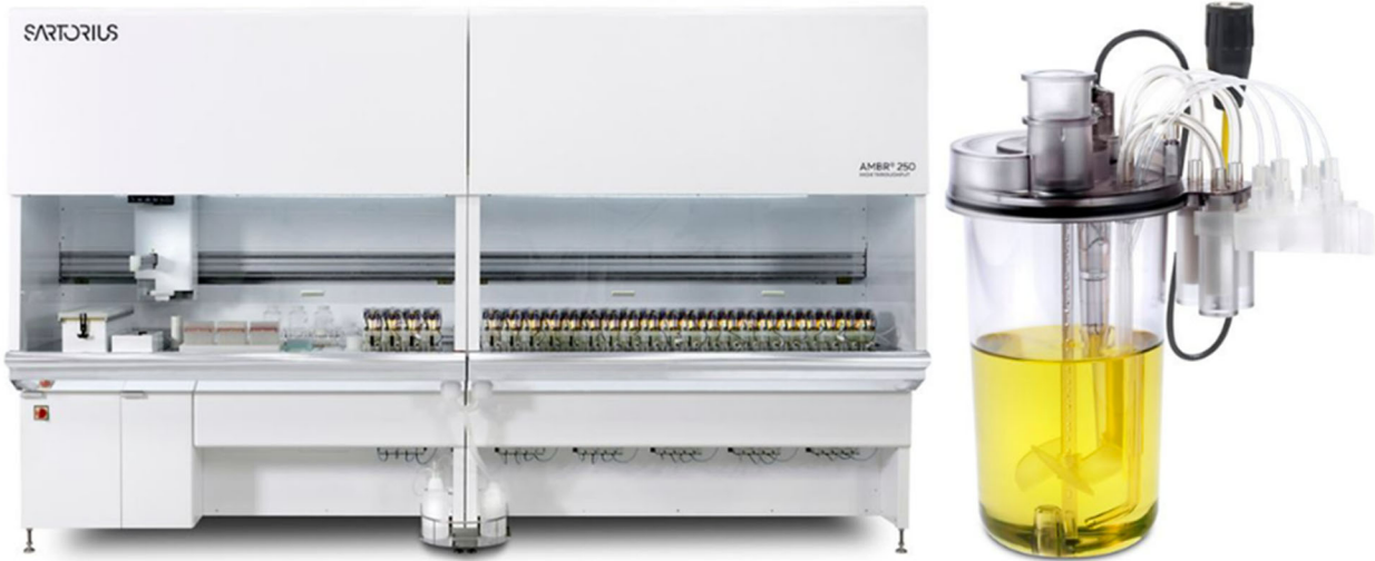
Figure 3: A Sartorius ambr 250 system and an enlarged individual, 250 mL disposable bioreactor that is part of the automated array. 24
