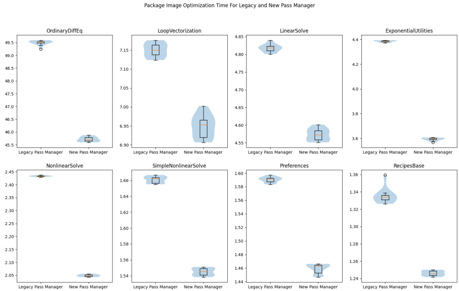
Figure 7-3: Pass Manager Timing Comparison for Package Image Construction Package images display a consistent reduction in time spent optimizing when using the new pass manager as compared to the legacy pass manager. Unlike figure 7-1, neither baseline nor scaling is consistent among subplots, due to small differences in large total optimization times.
