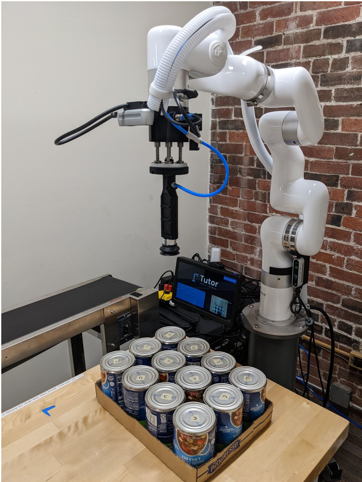
Figure B-2: Exploratory pilot study test setup with robot system, product, and conveyor belt.
