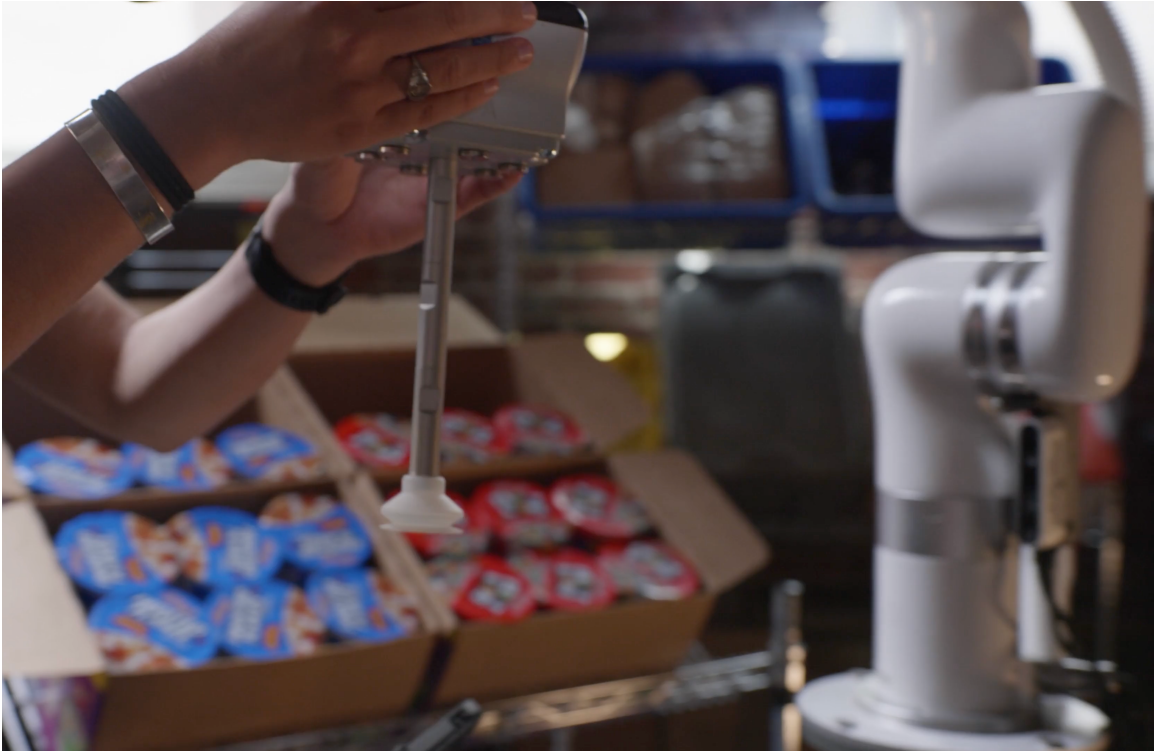
Figure B-1: Person moving collaborative Tutor Intelligence robot to the correct position.
