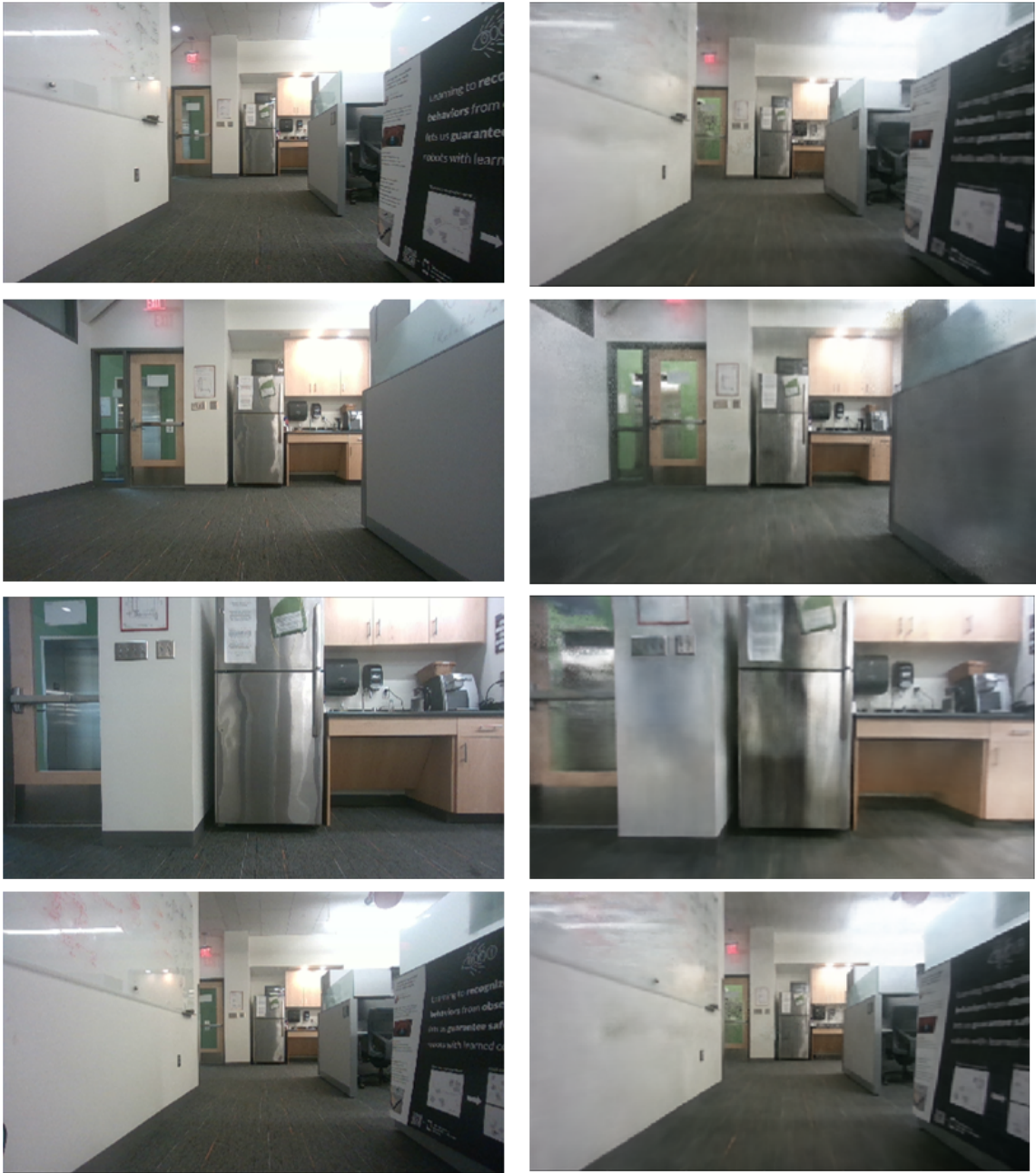
Figure 3-7: Left Column: true images viewed by the camera. Right Column: NeRF-rendered images using the pose estimate from Loc-NeRF. Images correspond to update steps number 20, 40, 60, and 100 which occur at 13, 20, 28, and 44 seconds into the experiment, respectively.
