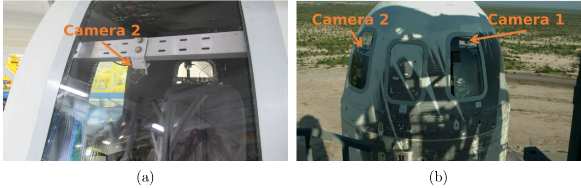
Figure 2-7: Cameras 1 and 2 mounted inside the New Shepard capsule looking out the capsule windows. Images courtesy of Blue Origin.
