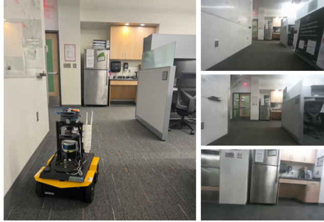
Figure 3-1: Real-time experiments with Loc-NeRF using a Clearpath Jackal UGV (left) equipped with a Realsense d455 camera. Examples of NeRF renderings near the beginning, middle, and end of the experiment (right).
