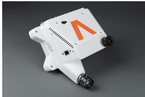
Figure 2-5: Draper Multi-Environment Navigator (DMEN) package: data collection package containing sideways and downward facing cameras, IMU, and logging computer.
