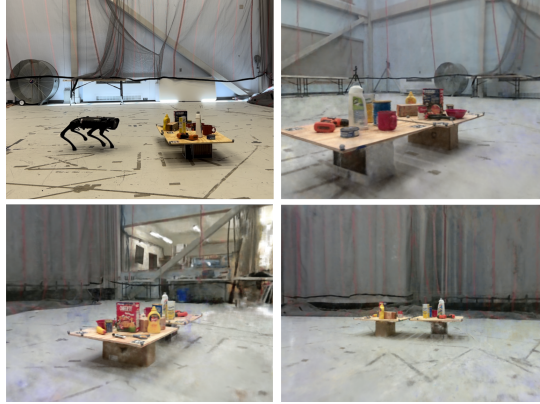
Figure 4-4: A1 quadruped rocket collecting monocular RGB data for NeRF training and VEF evaluation (top left). Three example NeRF rendered views using weights trained by camera data collected onboard an A1 robot.
