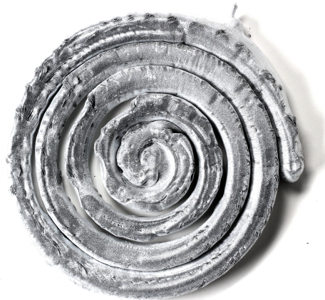
(a) 25mm Depth, 75mm/s, 20mm Pitch
