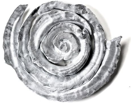
(a) 25mm Depth, 75mm/s, 20mm Pitch
