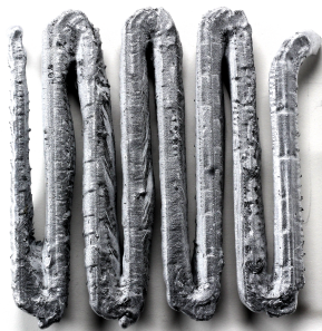
(b) 12mm Depth, 75mm/s, 20mm Spacing
