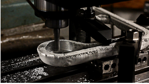
(a) Machining a Smooth Bore
