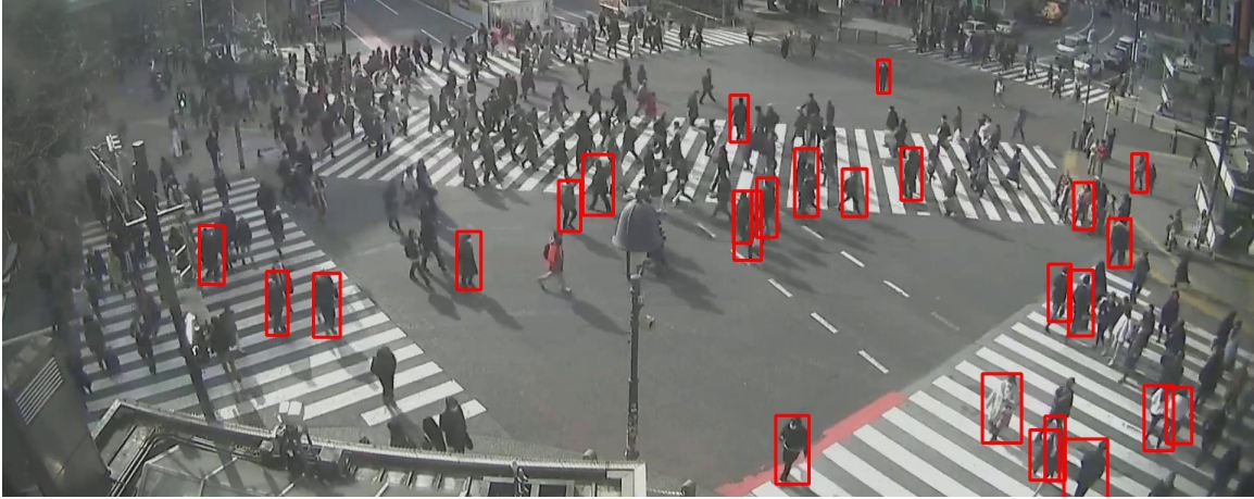
Figure 3-1: The results of a state-of-the-art object detection algorithm (filtered to “person” class) on one frame of urban . The algorithm misses 76% of individuals in the frame, but is still able to produce a conservative bound on the maximum duration of all individuals (Table 3-1).
