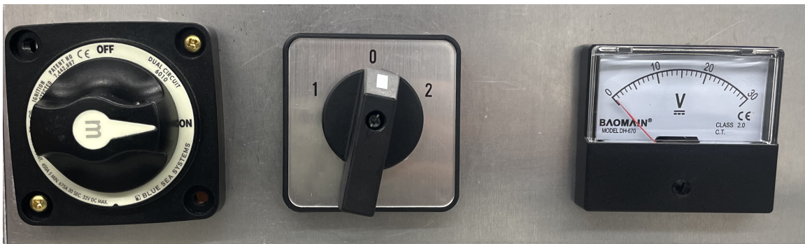
Figure 4-10: The pulse box's control panel. The black on/off switch connects and disconnects the box from the circuit, the silver 1/0/2 switch controls the capacitor's ability to charge and discharge, and the voltmeter reads the capacitor's voltage.
