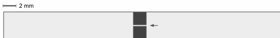
Figure 3-1: A drawing of a bridged HTS tape. The dark gray areas have been etched by the laser, creating a bridge of pristine REBCO.
