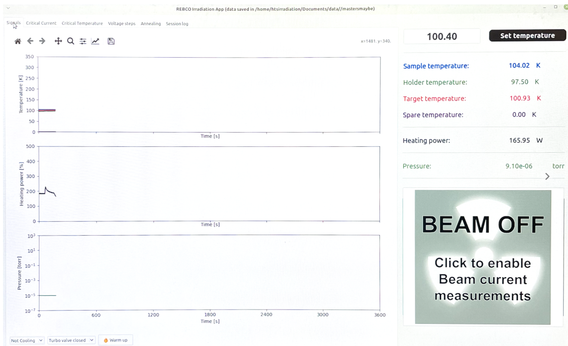
Figure 4-1: The graphical user interface (GUI) displaying the observed environment. The temperature is measured in the Cernox sensors in the target cryohead, sample holder, and on the sample, the pressure is measured in the vacuum chamber, and the heating power refers to the wattage of the heaters and coolers attached to the chamber. The temperature can be set from the GUI and the beam off button lifts the Faraday cup. The other GUI function utilized in this experiment is the critical current measurement.
