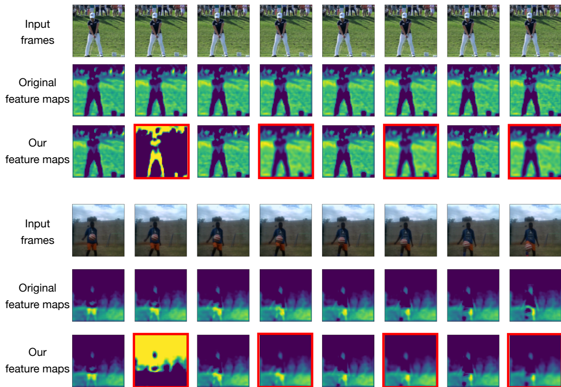
Figure B-2: Visualization of temporal-wise feature maps. We plot the temporal feature maps which are fully computed by the original convolution and those mixed with cheaply generated feature maps. The feature maps marked with red bounding boxes are cheaply generated. We do this analysis on 8-frame dynamic R(2+1)D-18 pretrained on Mini-Kinetics-200. These feature maps are the output of the first spatial convolution combined with ReLU non-linearity inside the ResBlock_1 . We can see that most of the cheaply generated feature maps looks no difference from the original feature maps, which further support our approach. Best viewed in color.
