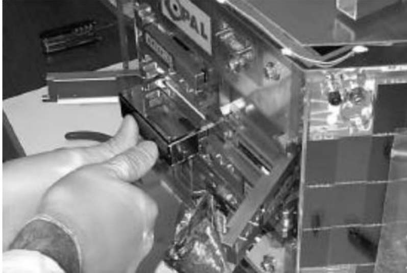
Figure 2-1: A MEMS PicoSatellite being loaded into a spring-loaded deployer on the OPAL spacecraft [29]
