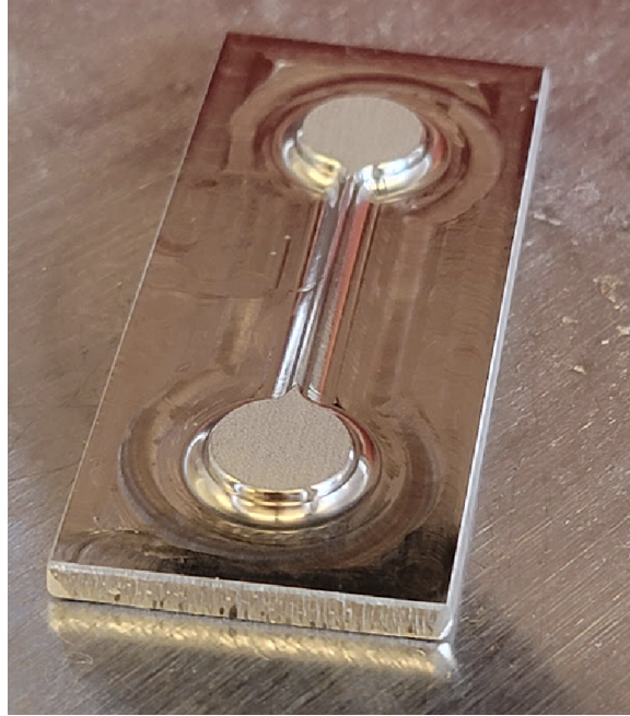
Figure 5-2: A CNC milled steel positive microchannel device used to stamp softer metals.
