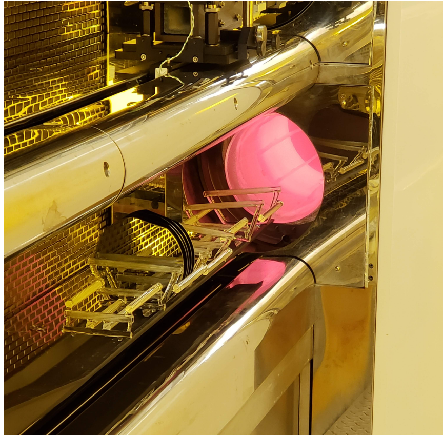
Figure 5-18: Wafers entering a furnace for thermal oxide growth. The quartz holder is needed to withstand the hot environment.
