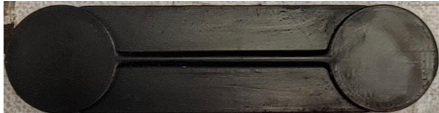
Figure 5-5: A 3D printed ABS plastic variant of the milled tool steel microchannel device.
