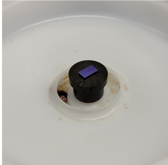
Figure 5-23: Silicon microfluidic device after spin coating with a fluoropolymer solution.
