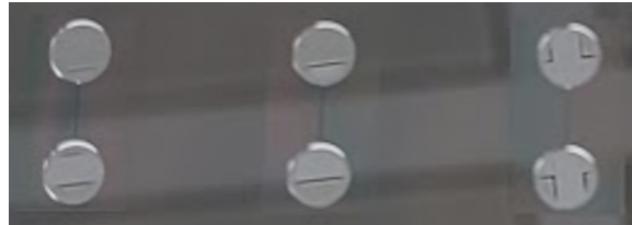
Figure 5-14: Grayscale exposure photoresist mask atop a silicon wafer. Devices are 100 micron wide microchannels 5mm long with two 5mm diameter reservoirs at either end.
