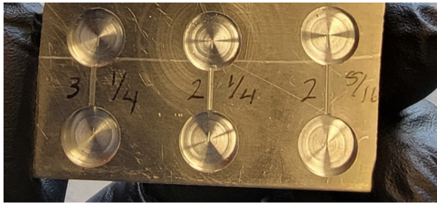
Figure 5-1: Several milled microchannels in an aluminum bar prior to sawing into individual devices.
