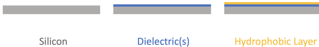
Figure 5-24: Fabrication cross-section evolution of the electrowetting test chip.
