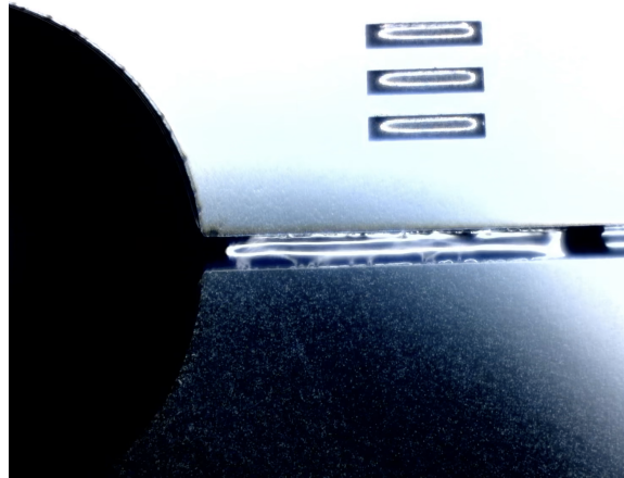
Figure 9-12: EMI-BF4 undergoing SCF into a plasma-treated fluoropel coated channel. Channel width is 100 micron and depth is approximately 300 micron. Note the clear meniscus pinning along the sharp ledge of this particular device.
