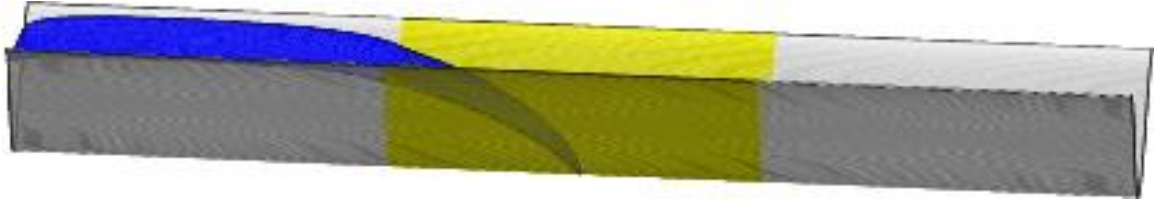
Figure 4-17: A rounded open microchannel with a hydrophobic region located in the central region (yellow) and hydrophilic regions on either end (gray.)
