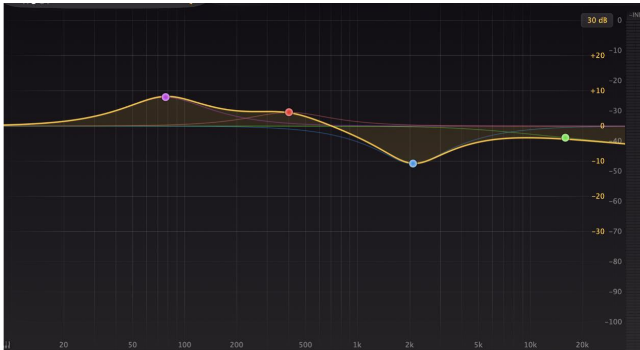
Figure 16: EQ from fabfilter Pro-Q 3. The image shows a graphic equalizer used to accentuate resonant frequencies in the process of finding resonant frequencies in the Uróboros.
