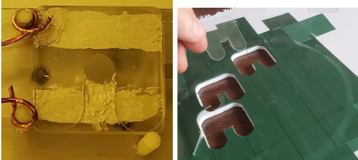
Figure 6-15: (Left) Glass holder showing the glass wafer, glass blank, steel electrode, and silver conductive adhesive traces. The three ceramic posts position the glass holder with preload from a flexure. The ceramic two posts on the left are coated with conductive adhesive, which make electrical contact to the glass holder. Wire wraps around the posts to supply voltage to the setup. The total resistance of each path is a few Ohms. (Right) Waterjetting setup for the glass wafer. The wafer is taped on sacrificial plastic sheet. The waterjet pierces the plastic and then cuts into the wafer.
