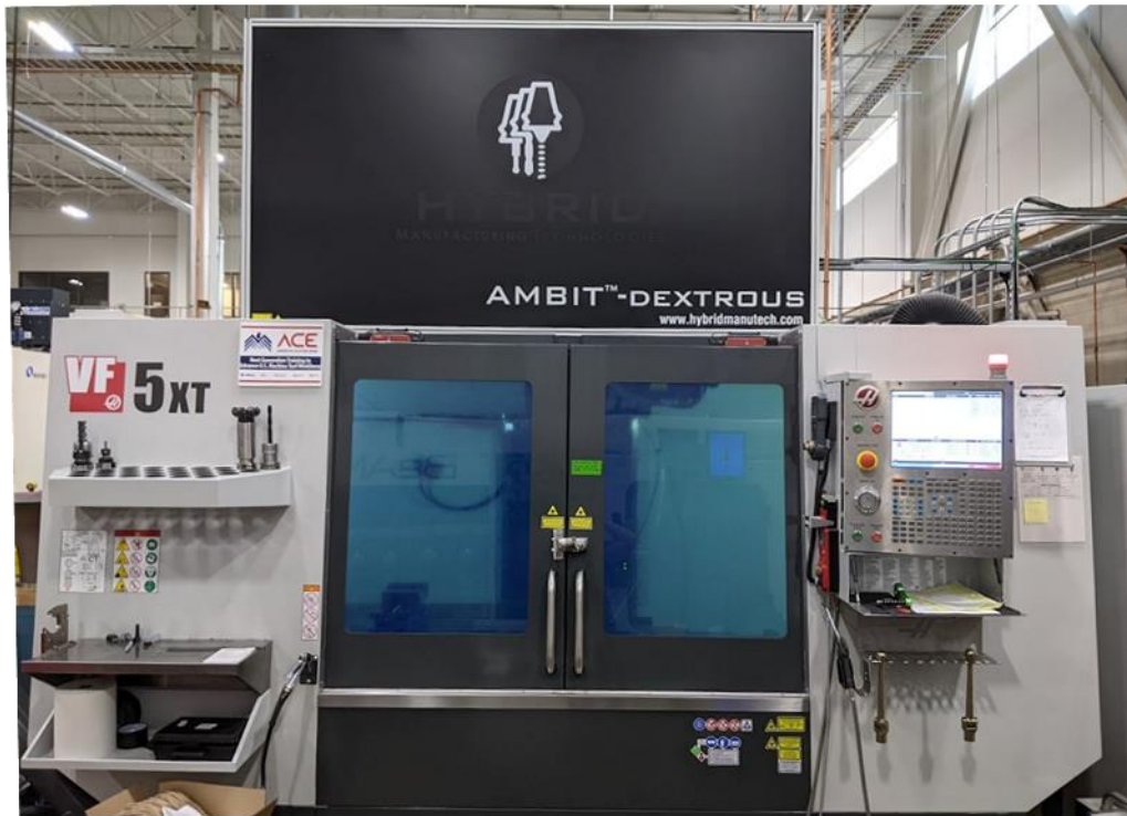
Figure 19: The Haas VF-5/40XT modified by Hybrid Manufacturing Technologies with blown-powder DED and polymer extrusion AM capabilities.
