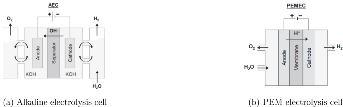
Figure 2-2: Conceptual diagrams of two types of electrolysis cells. Figures from Schmidt et al. (2017)
