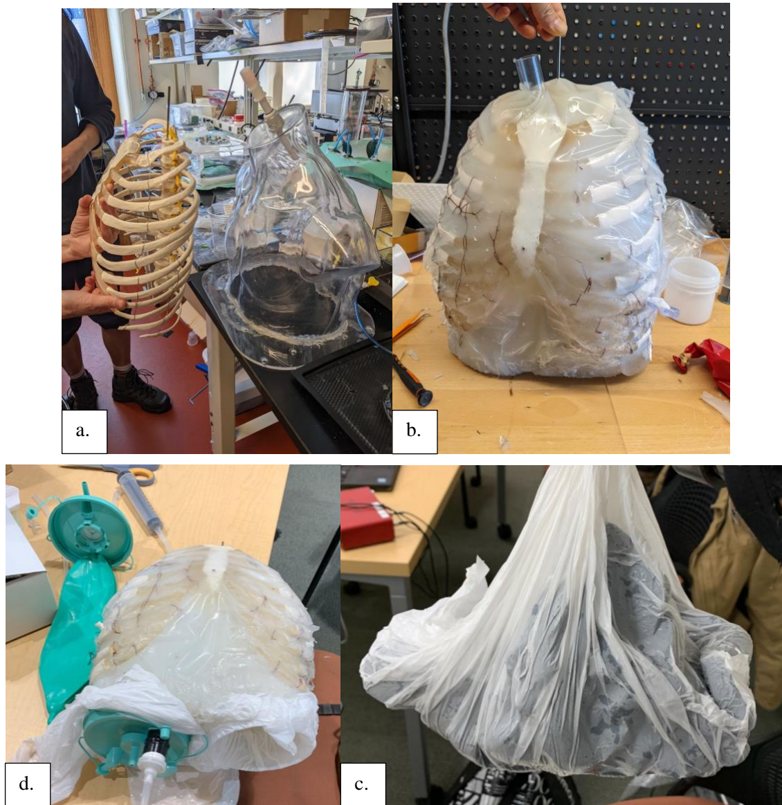
Figure 3-1: (clockwise from top left) a) The plastic skeleton model and chest mold used to cast the EcoFlex and Dragon Skin silicone rubbers. b) The completed phantom mold with internal pleural cavities included. c) The damp acoustic foam used to simulate lung tissue. d) The phantom with one complete lung, showing the anesthesia bag to be inserted into the second pleural cavity to allow for inflation of a pneumothorax.
