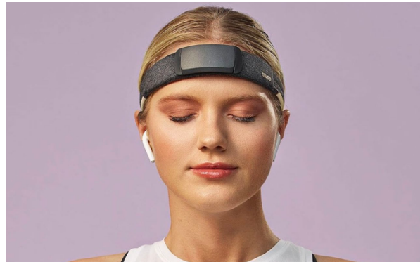
Figure 1. Muse, a “smart” headband that comes built-in with EEG brain sensors. The company allows the user to be able to interact with the live data after being filtered with their classification algorithm through a friendly user interface [4].
