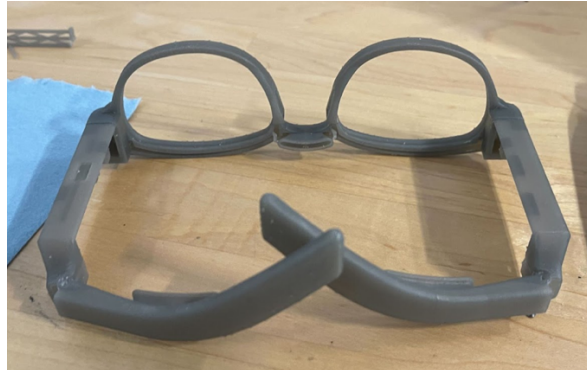
Figure 10. Frame assembly of glasses #028 with arms folded. Wires were attached with slight slack. After fully assembled, the lower half of the arms can close past 90° from vertical.
