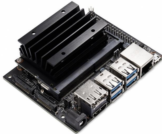
Figure 5-6: This image depicts the Jetson Nano Developer Kit used on the mobile robot
