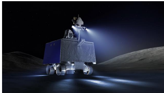
Figure 1-1: NASA’s Volatiles Investigating Polar Exploration Rover, or VIPER, is a mobile robot that will soon be used for resource mapping of the moon, mars, and beyond in preparation for human exploration.
