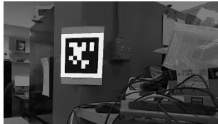
Figure 1: An AprilTag detection example. The detection program overlay highlighted tag image on the whole image after the tag is detected.
