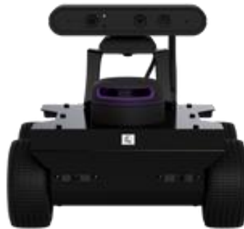
Figure 2-1: ROSbot 2 Pro, an autonomous robot platform with a sensor package and CPU conducive to a variety of jobs
