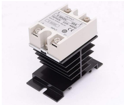
Figure 5-5: Shown in this figure is a 5-60V Solid-State Relay and Heat Sink.
