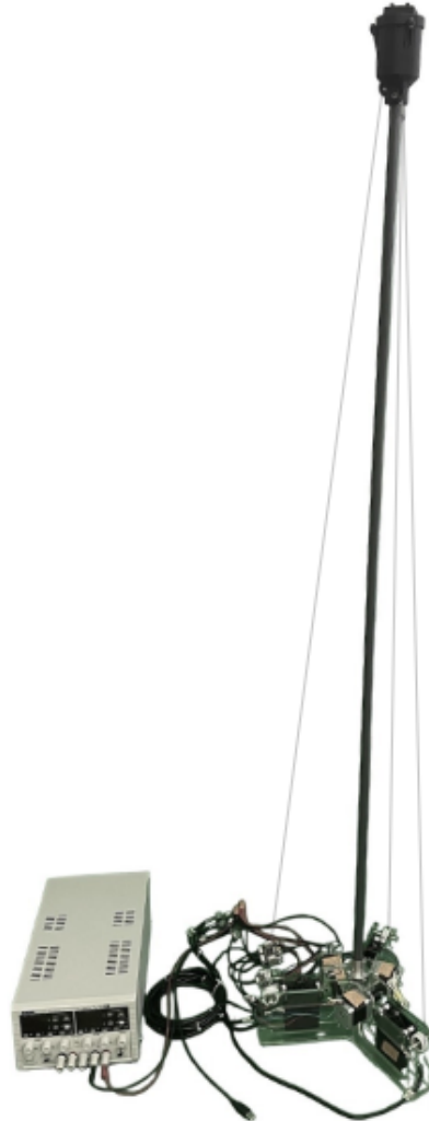
Figure 2-1. A photo of the scaled physical model. The stepper motor winches and load cells are located in the acrylic base, and the mock payload is screwed onto the tip of the PVC pipe. The IMU is mounted to the top of the mock payload, and its cable is wired through the pipe. The steppers are powered by a DC power supply.
