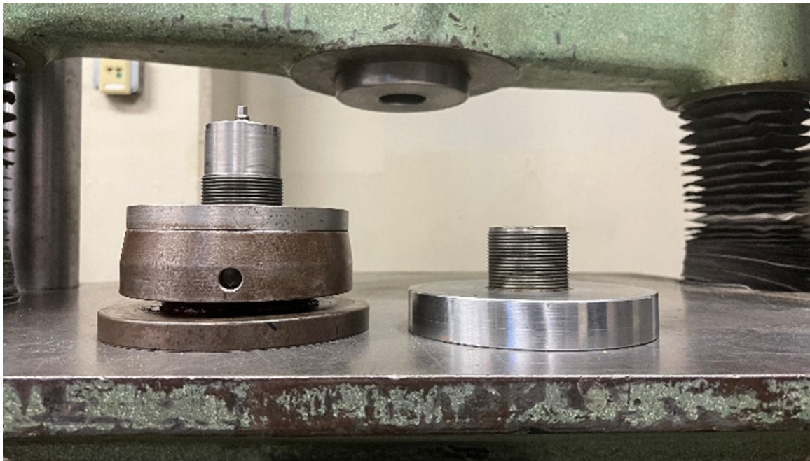
Figure 3-10: Photograph of flexible (left) and fixed (right) compression platens.
