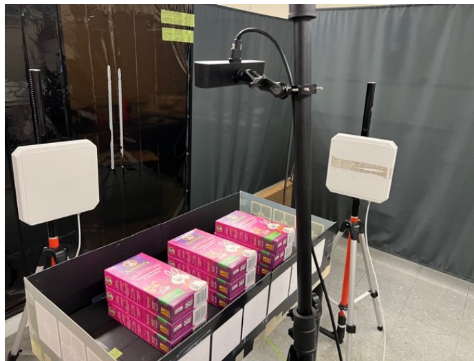
Figure 2-2: Placement of Zed 2 camera above the tested area
