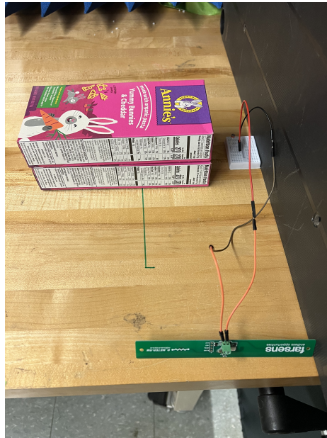
Figure 6-29: Situation when two stacks of boxes are placed in front of the photoresistor
