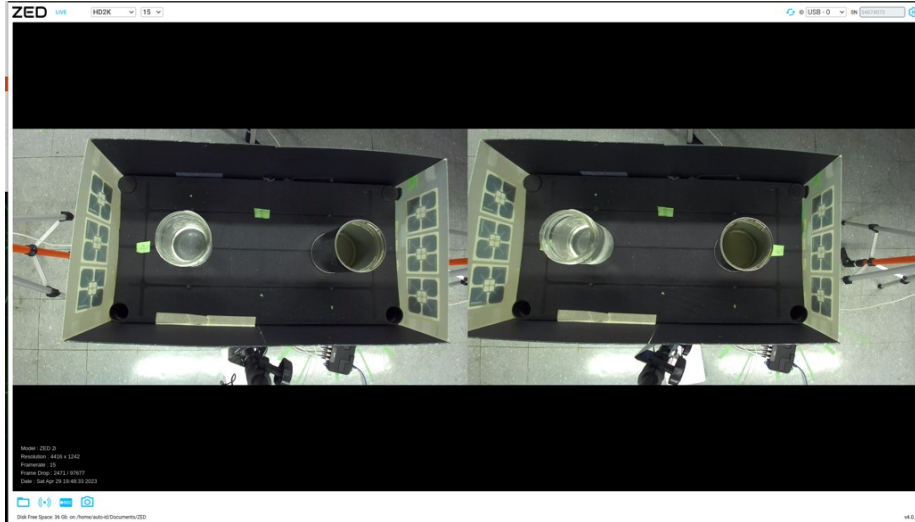
Figure 2-4: Camera view when one metal can (right) and one glass can (left) are put in the area
