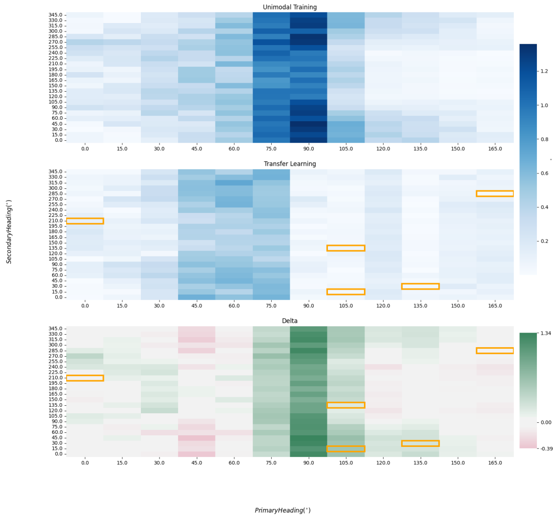
Figure 4-6: Primary vs Secondary wave heading angle pitch error: Unimodal Training and Random Transfer Learning.
