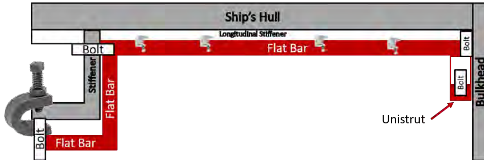
Figure B-5: Schematic of lower bar and mounting points.
