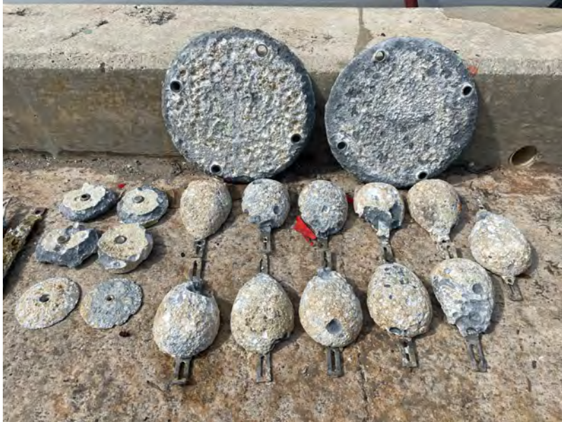
Figure 1-7: Bow Thruster and Propeller Zinc Anodes removed 1 year after installation
