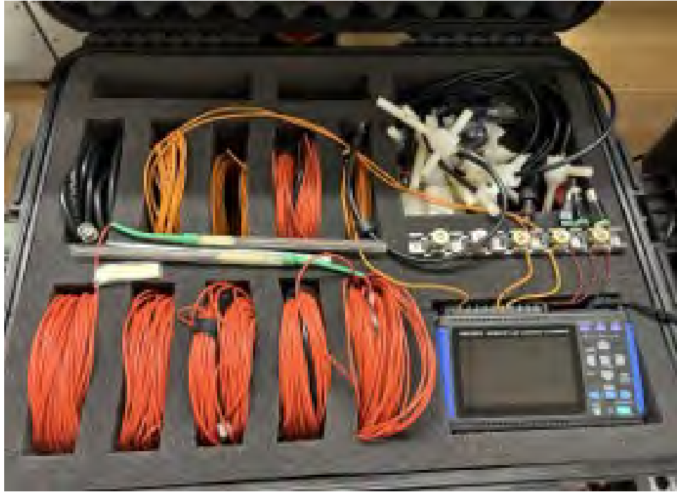
Figure 3-4: Hioki Data Logger with Cable Entries
