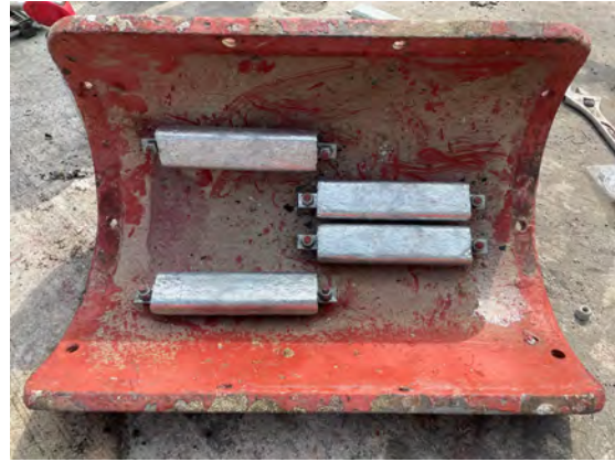
(b) Newly Installed Zincs
