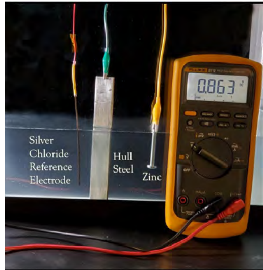
(b) Beaker Experiment with zinc anode
