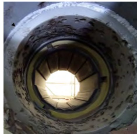
(b) Wide view of sand blasted bearing housing.
