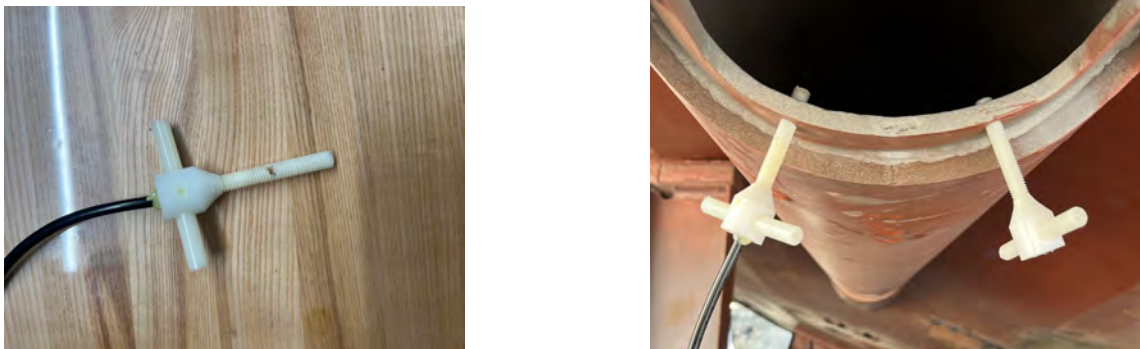
Figure 3-1: Temporary Custom Reference Electrodes
