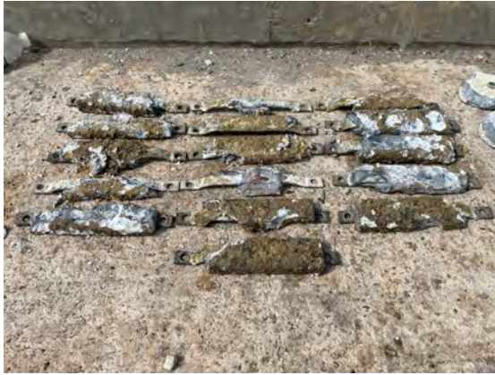
(a) Old zinc anodes after one year of wear.
