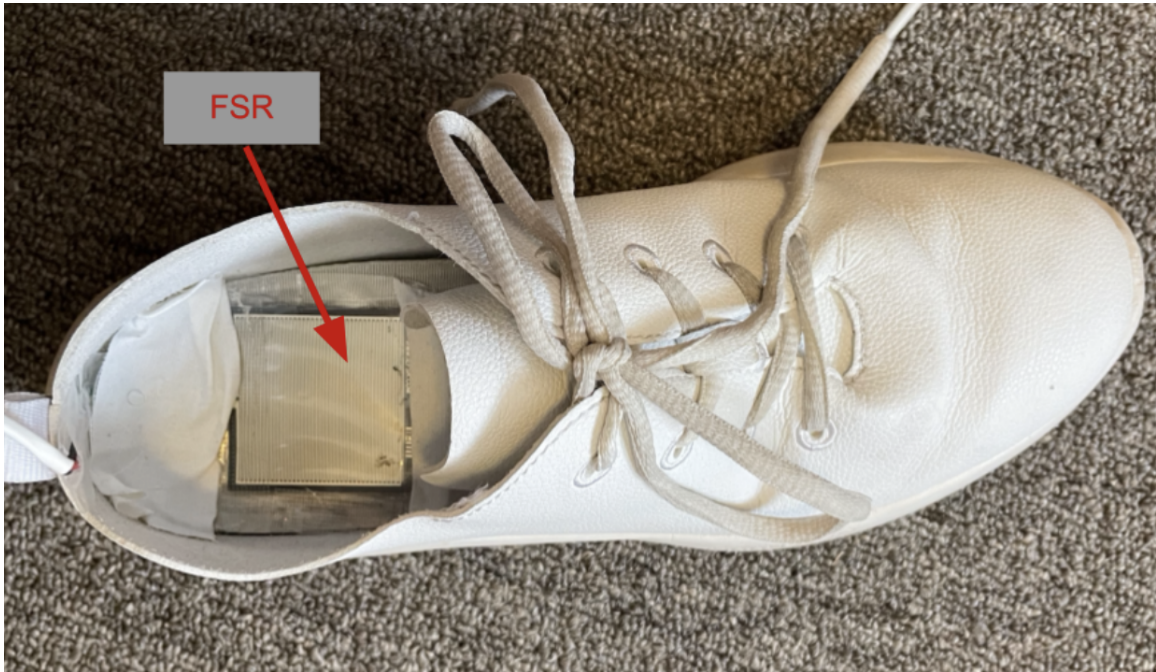
Figure 2-1: FSR attached to the heel of the shoe.
