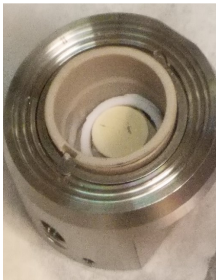
Figure 11. Picture of S50 sample pellet after accidental contact with a piece of lithium metal foil during the test cell assembly process in a glove box. Area of contact almost immediately changed color from cream to black.
