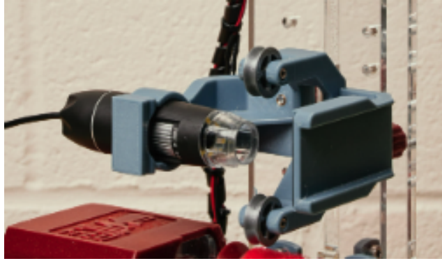
Figure 24. Camera based diameter measurement system
