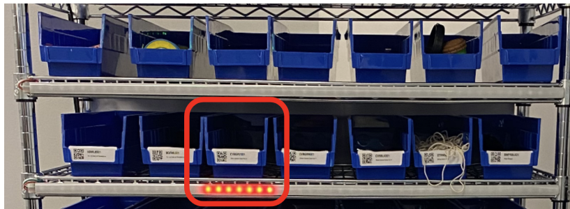
Figure 117. LED indicating bin position
