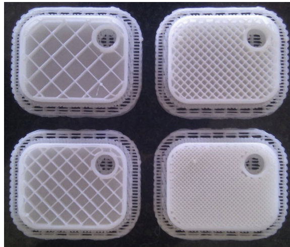
Figure 71. Infill Density in Extrusion 3D Printing [31]
