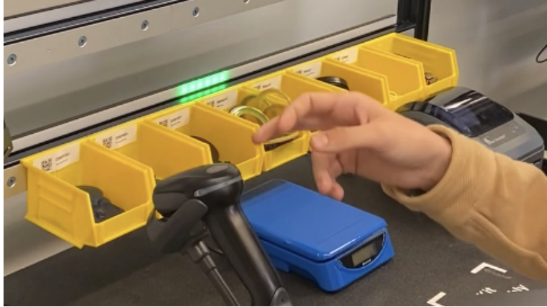
Figure 113. LED guiding worker to pick parts
