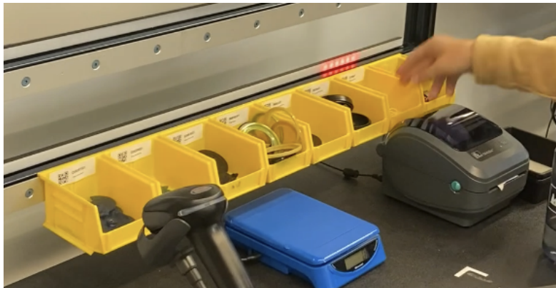
Figure 114. LED alerting worker picking wrong part
