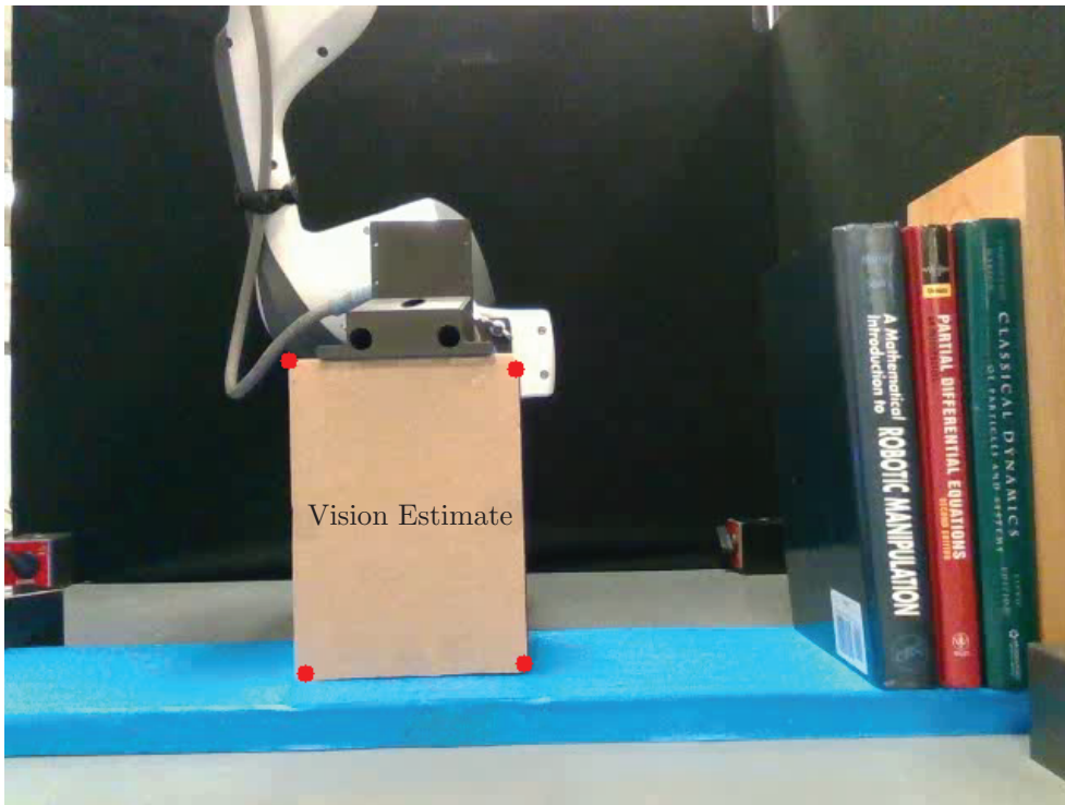
Figure B-7: The final result is an estimate of the corner locations of the object.
