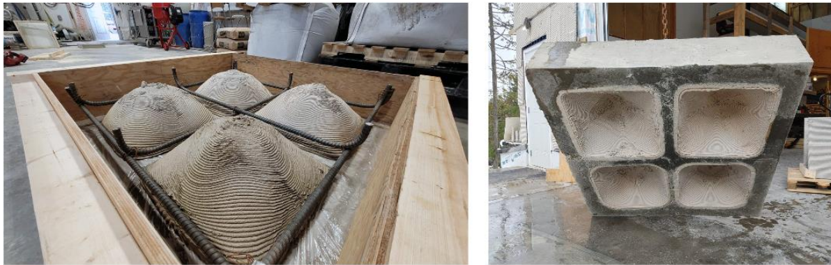
Figure 5-14: Proof of concept for fabrication of flat concrete element with conventional rebar and fabrication methods, and additively manufactured formwork that can be sized according to optimal dimensions for slab
