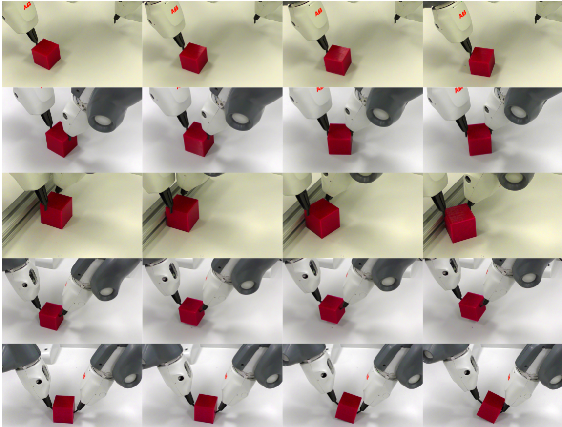
Figure 3-7: Experimental validation of our model Our optimized behaviors can be applied for real world execution, snapshots of each open-loop experiment are shown (each blue box corresponds approximately to the goal pose of the object). Top to bottom: 1) transversal pushing with a desired angle. 2) Rotating 45^\circ in-place. 3) Transversal pivoting against a wall. 4) Grasping vertically. 5) Sagittal pivoting.
