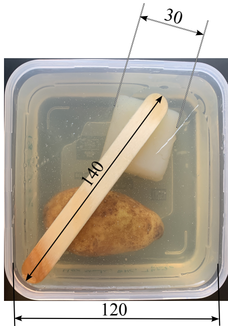
Figure 5-1: The ultrasound phantom fabricated for testing and validation
