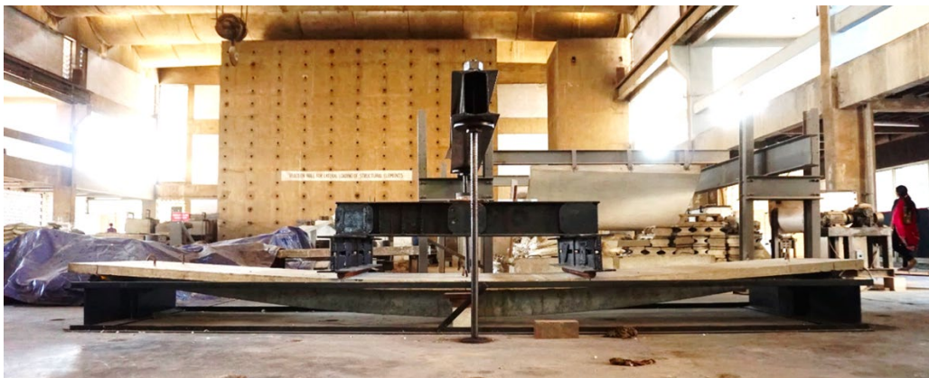
Figure 4. Formwork (top) and load testing setup (bottom) of the prototype shaped ribbed slab (Ismail & Mueller, 2021). Both images were shown to survey participants.
