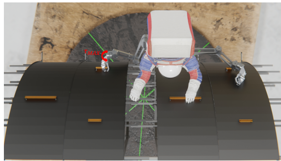
Figure 2-6: Maximum torque vector (at the wrist joint of the SuperLimbs).
