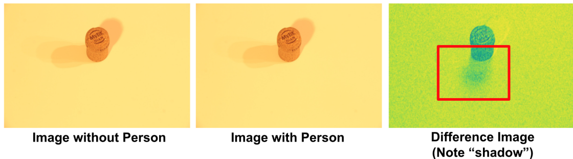
Figure 3-1: Two images of a cork were taken with and without a person standing just out of view of the camera. The person did not cast a visible shadow on the scene, and there is no obvious difference between the two images. However, when the image without the person is subtracted from the image with the person, a difference image shows a clear "shadow," as if the person were an illumination source. While subtle, these cues are detectable and can be explained using the principle of differential imaging.
