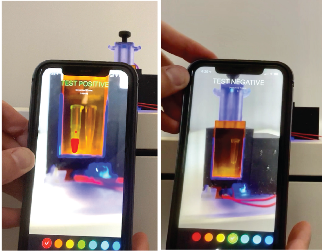
Figure A-3: Adjunctive mobile phone application supports automated quantitation and result interpretation.
