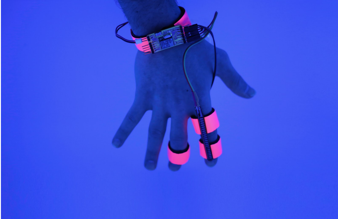
Figure 23. The Dormio PCB and handworn system, dorsal side. Flex sensor is visible on the pointer figure. Photo credit Oscar Rosello
