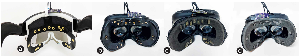
Figure 2-4: The image depicts every headset variation explored during this research. a) AR headset with flexible PCB & gold plated electrodes. b) VR headset with flexible PCB & gold plated electrodes. c) VR headset with hydrogel electrodes. d) VR headset with Ag/AgCl electrodes.
