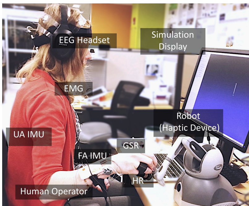
Figure 1-1: Subjects interacted with the virtual task by controlling a robotic interface (i.e., haptic device). Physiological response (e.g., EEG, GSR, EMG) and user kinematic movements were recorded from wireless inertial measurement units (IMUs) on the upper-arm and forearm, as well as encoder readings from the haptic device. Image by Wang et al.
